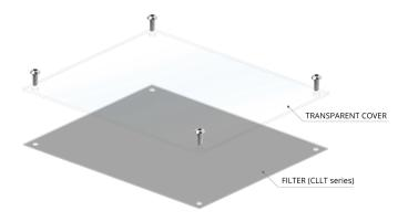
Additional protective window, togheter with its fixing screws, is supplied with the filter
